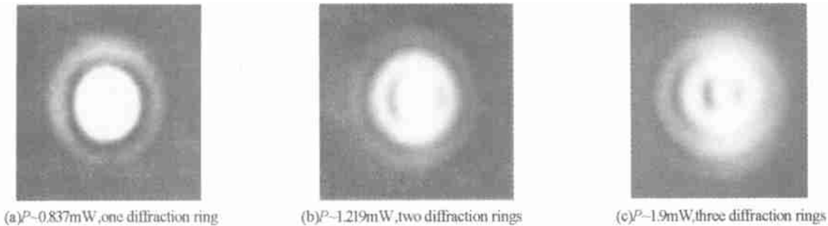
图 4 光克尔效应引起的衍射环 Fig. 4 Diffraction rings caused by Kerr effect
